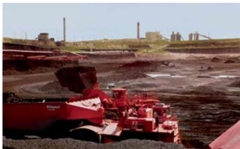
A loader fills an end dump truck in the pit of the Wyodak Mine in the 1990s. In-pit equipment continued to grow in size and capacity as mining technology progressed.
