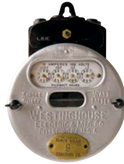
Westinghouse Type C 1906-1911. The first known patent for an electric meter was issued in 1872. While the look of the basic meter has evolved, the function remains the same: to measure the use of power.
